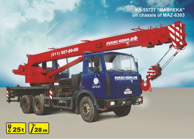
The mobile crane **KS-55727 "Masheka"** on chassis of **MAZ-6303**.
