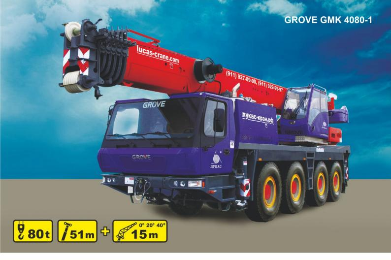
The **GROVE GMK 4080** mobile crane with a lifting capacity of **80 tons** and a boom of **66 meters**, is one of the most popular cranes of the **LUKAS-CRANE** company.
