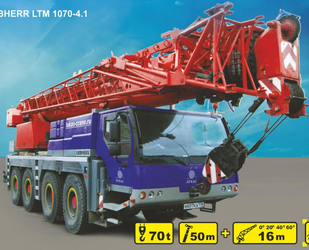
The **LIEBHERR LTM 1070-4.1** mobile crane with a lifting capacity of **70 tons** has a main boom of **50 meters** and a lattice jib of **16 meters**. Maximum boom reach **48 meters**.
